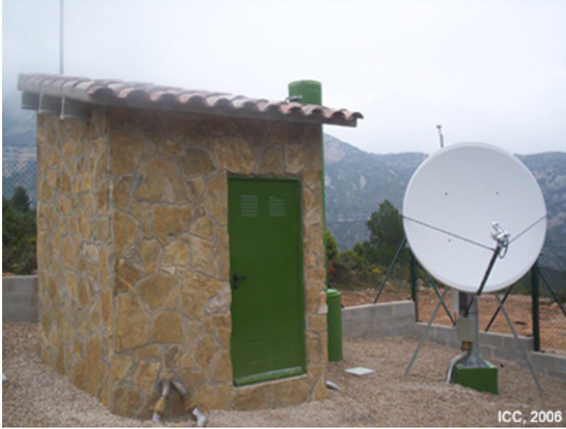
Detail of the instrumental house with the VSAT antenna and the geodetic pillar
